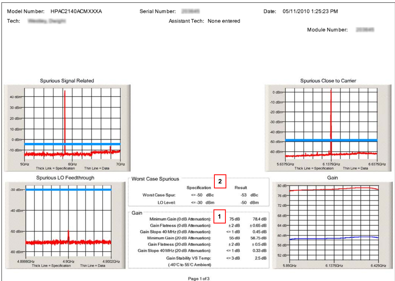
Figure 6-1: Spurious and Gain Data
