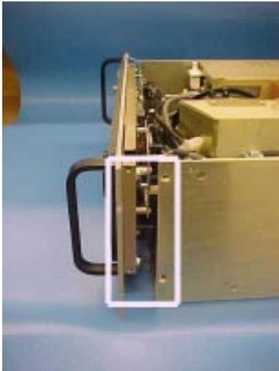
Place the TWTA onto a bench that can properly support the weight. Remove the D20161 front panel assembly screws, two on each side of the front panel. Once the screws are removed slightly pull the front panel assembly forward.
