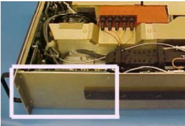
Place the TWTA onto a bench that can properly support the weight. Remove the four mounting screws from the right side wall.
