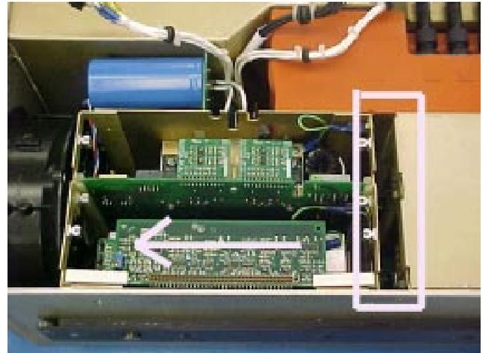
Slide the HVPS assembly to the rear of the TWTA as shown at the right until the HVPS disconnects from the PPM assembly.
