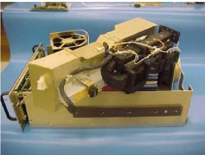
Replace the defective component using D30170-003-TAB assembly print as a guide. NOTE: If the TWT is being replaced, be sure to use heat conductive grease on the tube baseplate.
