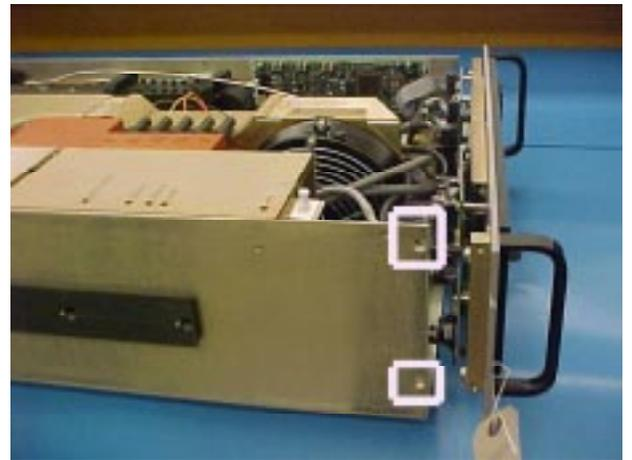
Remove the D20161 front panel assembly screws, two on each side of the front panel. Once the screws are removed pull the front panel assembly forward slightly to allow space to move the PPM assembly.
