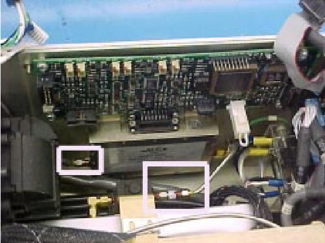
Disconnect the RF cable between the tube and SSA at the circulator on the tube input.
