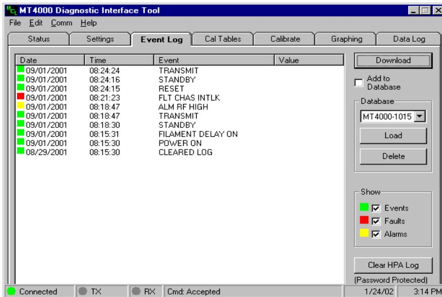
If the event/fault log is cleared before the failure is analyzer there is also a data log (shown below), which cannot be cleared and can only be accessed through the diagnostic interface. See TN4000-3 *Technical Note, Operation of MT4000 TWTA* for instructions on downloading the data log.
