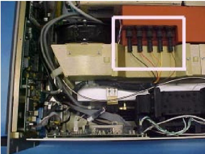
Disconnect the tube high voltage wires from the High Voltage Transformer & Filter Assembly (shown at the right). Be careful not to damage the insulation on these HV wires.
