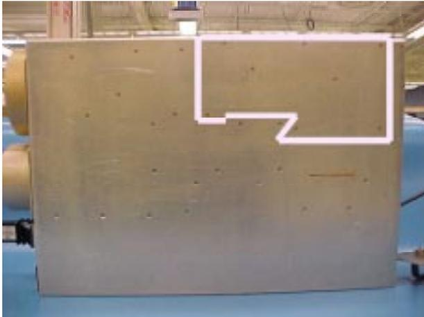
Place the TWTA onto a bench that can properly support the weight. In the box shown to the left are the screws that hold the PPM assembly in place. Remove the hardware for the PPM. Once the hardware is removed, place the HPA on a bench right side up. The assembly is not removable yet.
