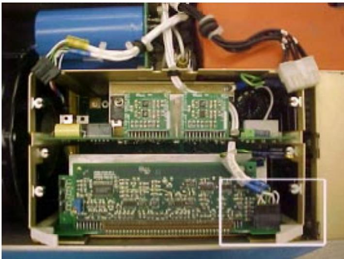
Disconnect the third connection (filaments) from the HVPS shown at the right.
