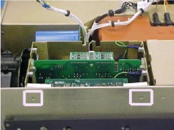
Remove the two screws on the side of the TWTA shown at the left.
