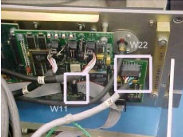
Disconnect W11 & W22 from the D20161 front panel assembly; these connect to the PPM.
