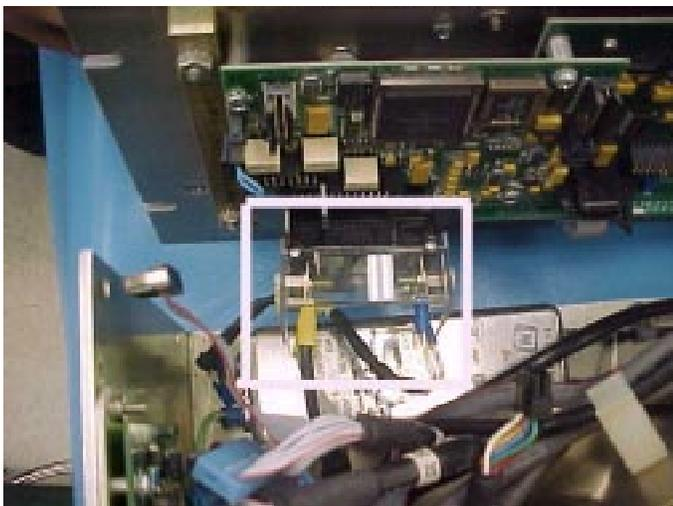
Disconnect the AC connection to the circuit breaker. You can now remove the Front panel assembly.
