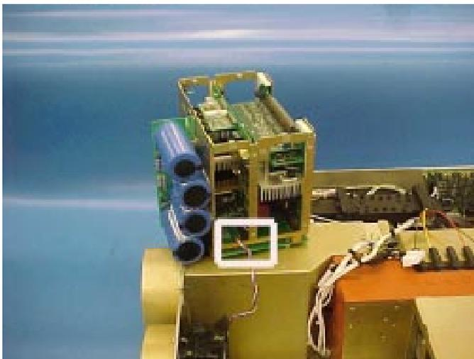
Once the HVPS assembly is disconnected from the PPM assembly, slowly lift it straight up and set it on the RF output assembly.
