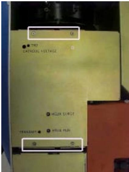
Place the TWTA onto a bench that can properly support the weight. Remove the four screws holding the top cover of the HVPS Field Replaceable Unit (FRU) Module & remove the cover.
