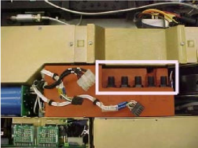
Confirm the high voltage tube leads are labeled correctly. Disconnect the high voltage tube leads from the high voltage connectors shown at the left.
