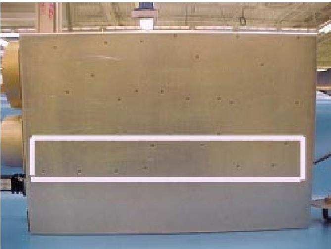
Place the TWTA onto a bench that can properly support the weight. In the box shown to the left are the nine screws that hold the RF output assembly in place. Remove these screws, once done place the HPA on a bench right side up. The assembly is not removable yet.
