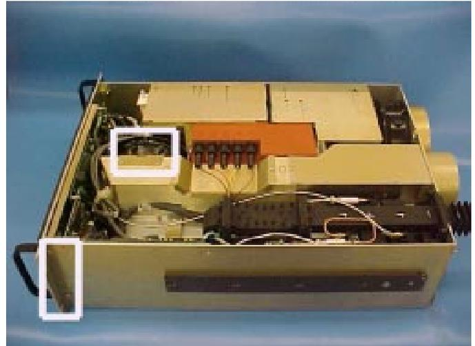
Open the cable clamp on the front of the plenum and remove the cables.
