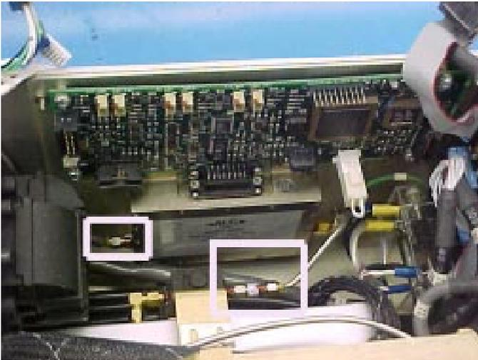
On the back of the HPA remove four waveguide mounting screws and two plenum mounting screws shown at the left. Disconnect and remove the RF input cable assembly.
