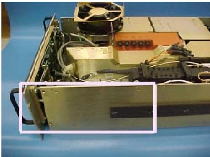
Flip the plenum blower up and on top of the PPM assembly.
