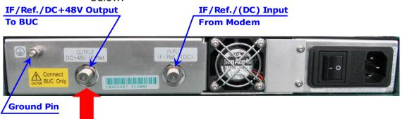
Connect the coaxial cable which connects to the BUC.
