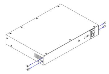
Step 2: Position the rack-mount flanges (Rack-mount Kit: No. 1) both sides of the Unit as shown in below.Install four M4X10mm flat head screws to flanges and the Unit.
