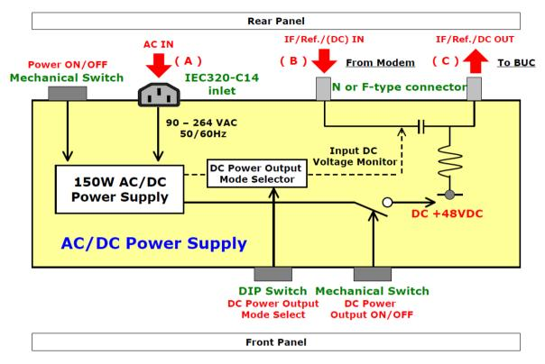
Schematic Diagram of Inside AC/DC Power Supply
