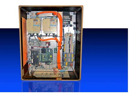
The ACS3000 controller provides three-axis control for antenna azimuth, elevation and feed polarization.
