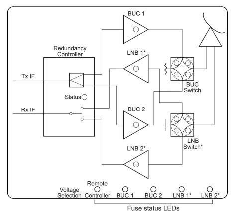
Figure 9: Control panel on the redundancy controller
