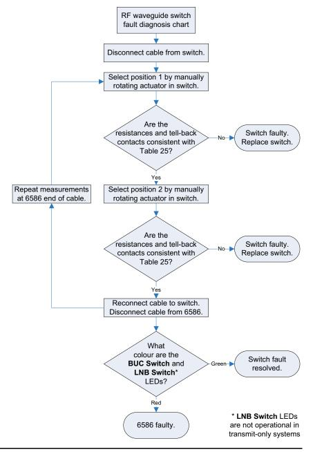
Figure 26: RF waveguide switch fault diagnosis chart
