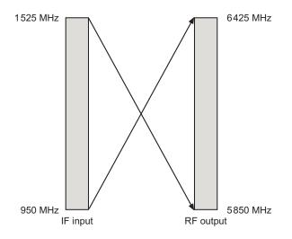
Figure 5: C-Band frequency conversion plan at an LO frequency of 7600 MHz
