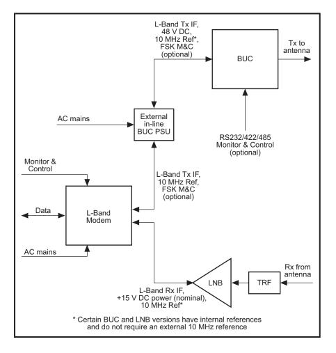
Figure 2: BUC with L-Band modem, external in-line PSU, and LNB
