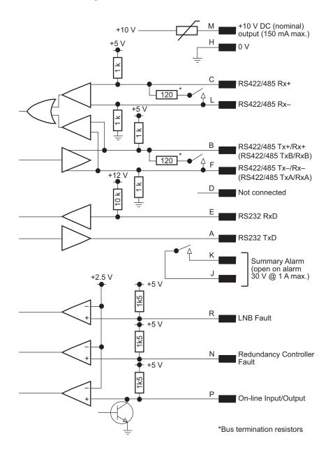
Figure 13: Monitor and control interface of the BUC
