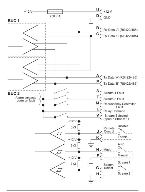
Figure 14: Auxiliary I/O interface of the redundancy controller
