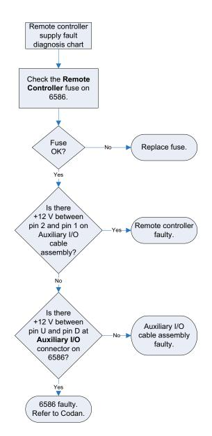
Figure 27: Remote controller supply fault diagnosis chart
