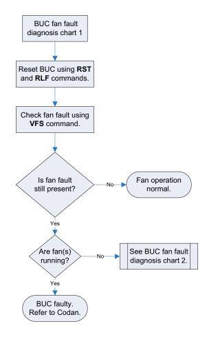
Figure 23: BUC fan fault diagnosis chart 1
