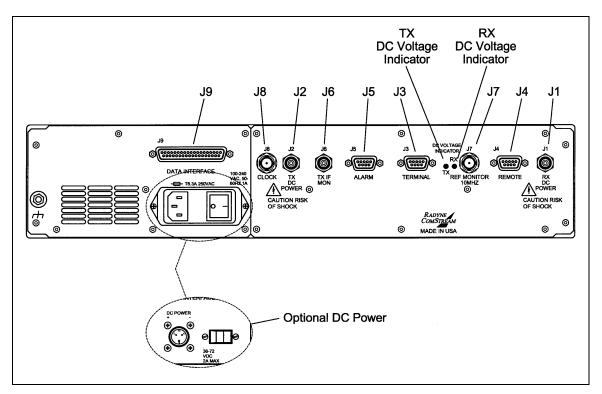
Figure 5-1. DMD2401 LB/ST Satellite Modem w/ RS-422 Data Interface
