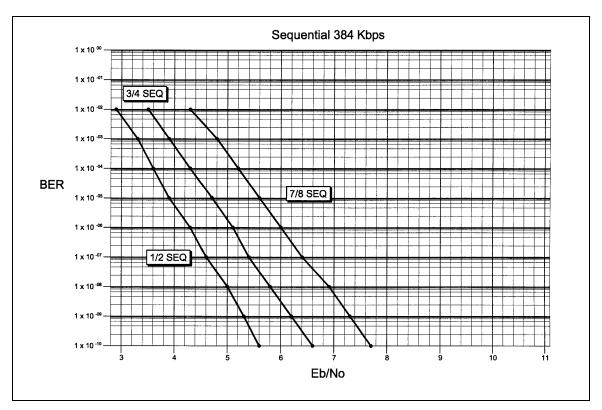
Figure 4-4. Sequential 384 Kbps BER Curve
