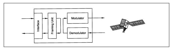
Figure 3-8. Tx/Rx Baseband Loopback
