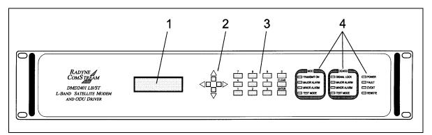
Figure 4-1. DMD2401 LB/ST Front Panel
