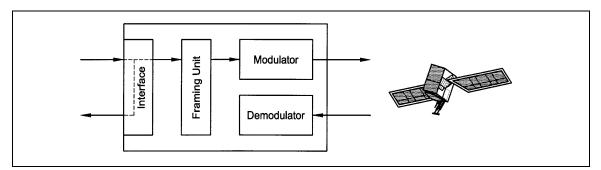
Figure 3-3. Tx Terrestrial Loopback
