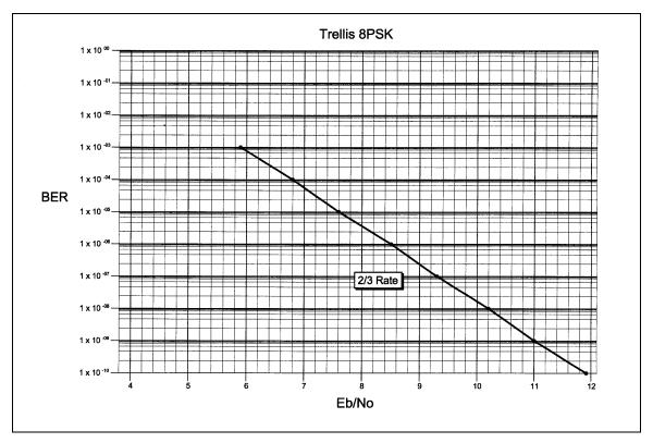
Figure 7-5. Trellis 8PSK BER Curve
