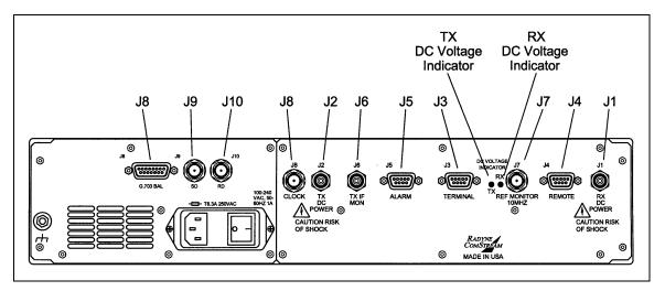
Figure 5-3. DMD2401 LB/ST with G.703 Data Interface
