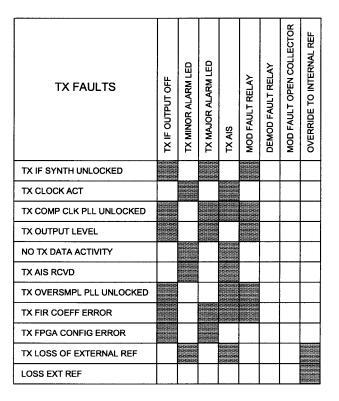
Note: When EXT EXC is used as a reference for the Mod Clock, and activity on the EXT EXC is lost, the modem switches Tx clock reference to SCTE if it exists, otherwise it switches to SCT.
