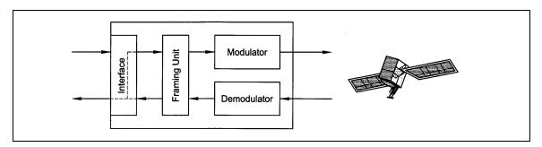
Figure 3-4. Rx Terrestrial Loopback
