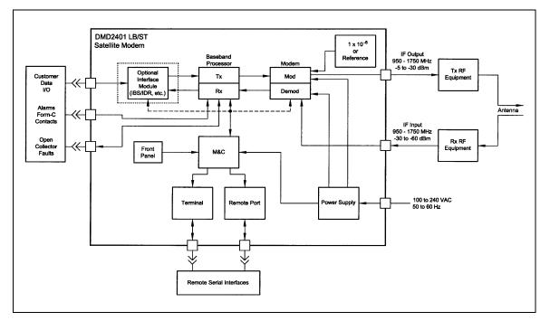
Figure 3-1. Functional Block Diagram
