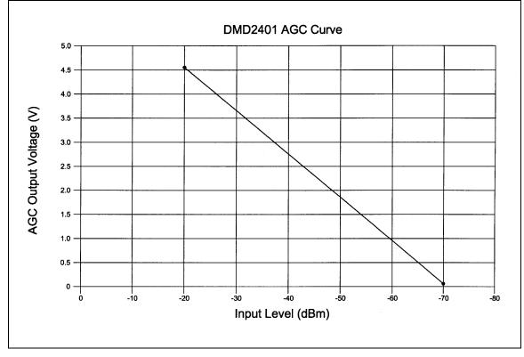
Figure 6-6 represents the AGC Curve for the DMD2401 LB/ST.
