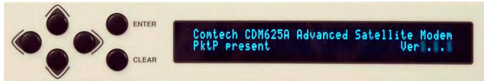
Figure T-2. CDM-625A Front Panel Keypad and Vacuum Fluorescent Display
