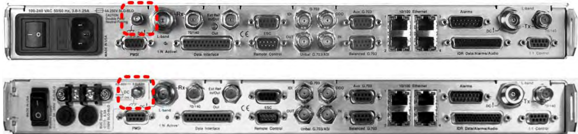
(TOP) Standard AC Chassis (CEFD P/N PL-0021325) (BOTTOM) Optional 48V DC Chassis (CEFD P/N PL-0021327)
