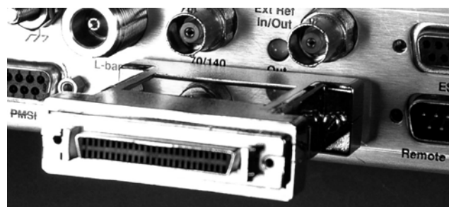
CIC-60 Interface Adapter Module (Installed, HSSI Interface Side Shown)
