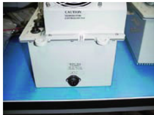
Figure 2-3. AC Power Connection.
