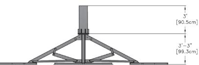
**Model:** PXL-2 EHD (3 Trays Per Leg) **Type:** Non-Penetrating Mount System
