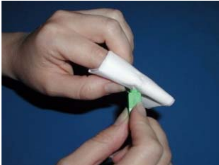
Figure 21 Wiping the connector with a Kim wiper
