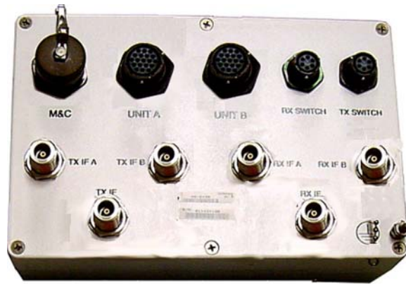
Figure-B-13. Remote Switch Box Assembly, AS/0490
