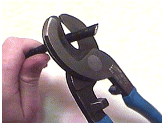
Figure 13 Coax Cable Cutting Technique
