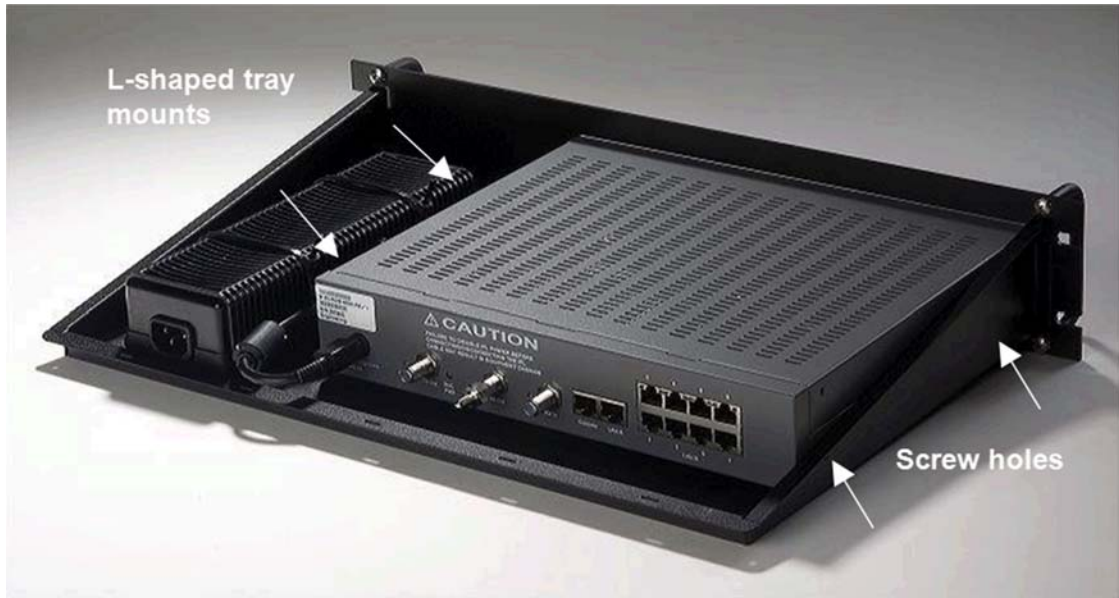
Figure 9 Rear View of an iDirect 5000 series™ Satellite Router in a Rack Mount Tray
