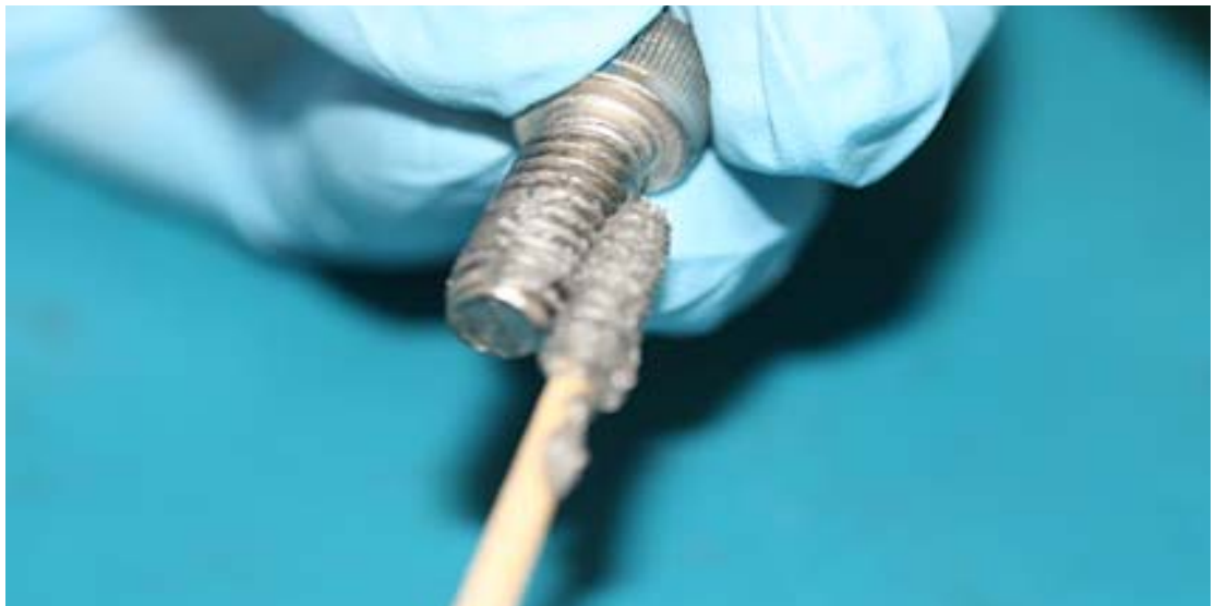
Figure 3.13 Applying the Anti-Seize Lubricant
