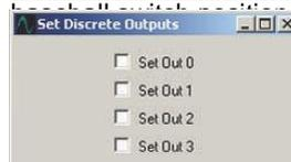
**Set Discrete Output[s]** – There are 4 general purpose discrete outputs 1-4. The user maps in software how they are used; 5V = set, 0 = clear. The rackmount controller reads back the state of each pin.
