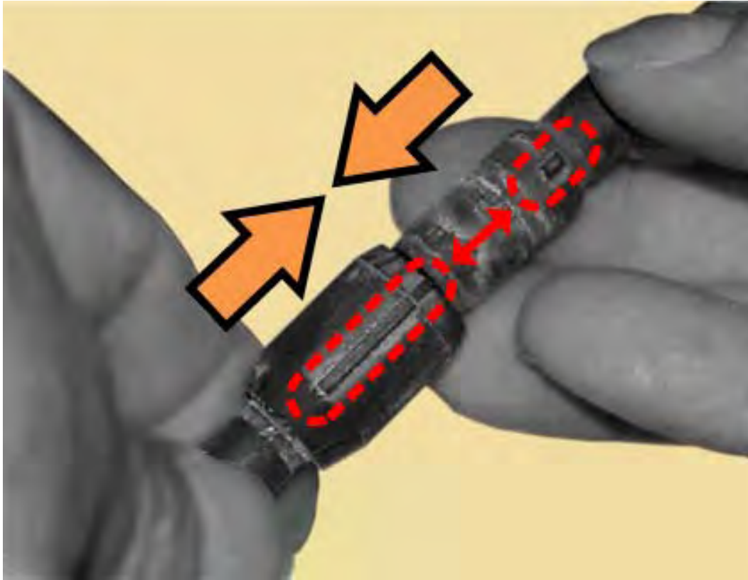
Figure C-17. Reconnect the Fan 1 / Fan 2 Power Supplies
