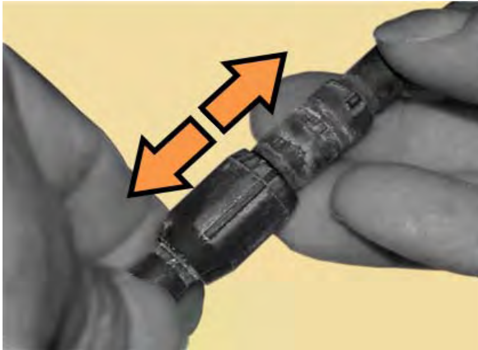
Figure C-15. Disconnect the Fan 1 / Fan 2 Power Supplies
