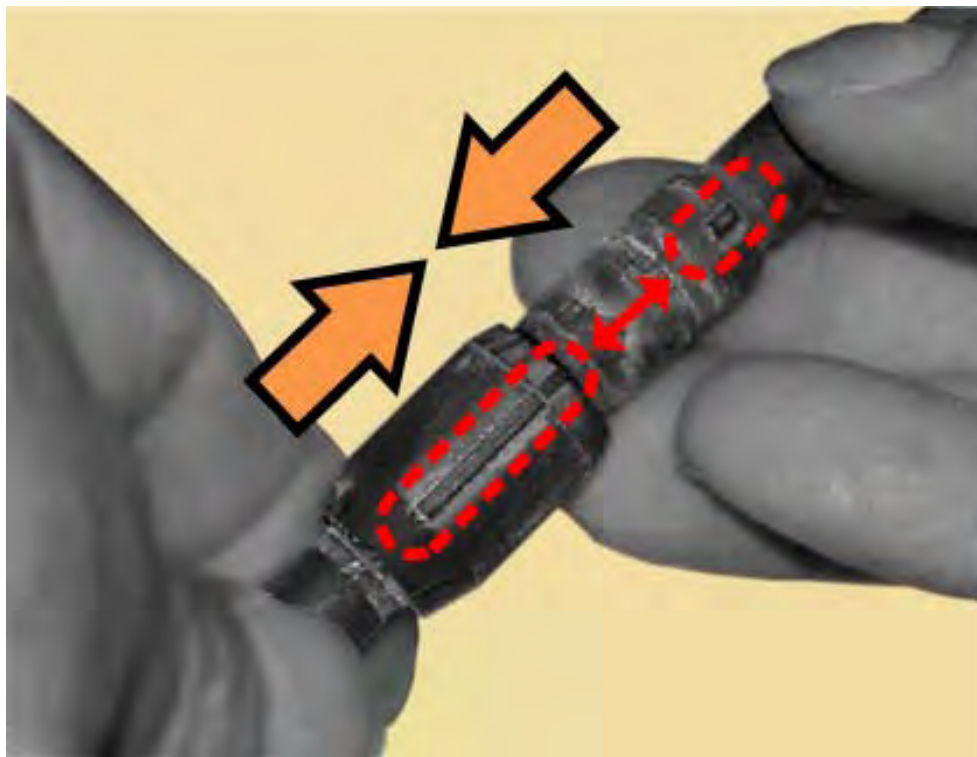
Figure C-12. Reconnect the Fan 1 / Fan 2 Power Supplies
