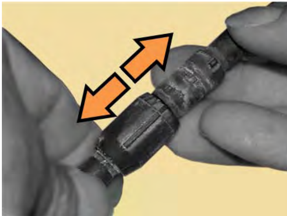
Figure C-10. Disconnect the Fan 1 / Fan 2 Power Supplies
