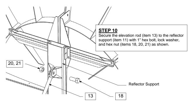
**Figure 14: Elevation Rod Assembly to Reflector Support**
