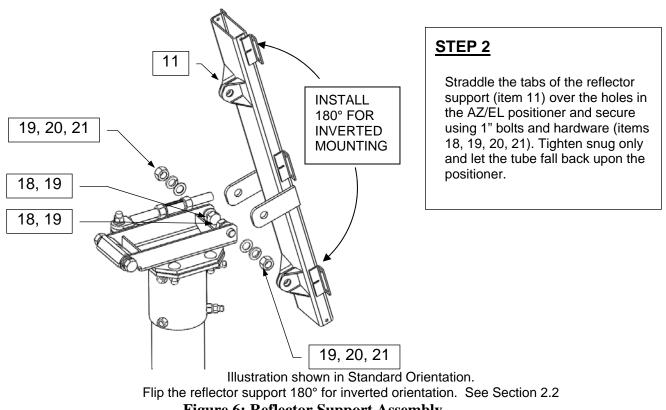
Figure 6: Reflector Support Assembly
