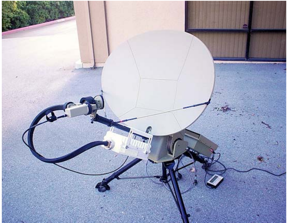
Figure 3.2 IBUC 2 Field Installation
