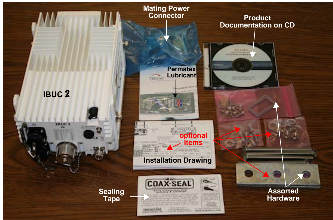
Figure 3.1 Contents of an IBUC 2 Shipping Carton
