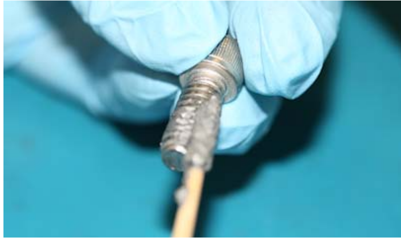
Figure 3.6 Applying the Anti-Seize Lubricant
