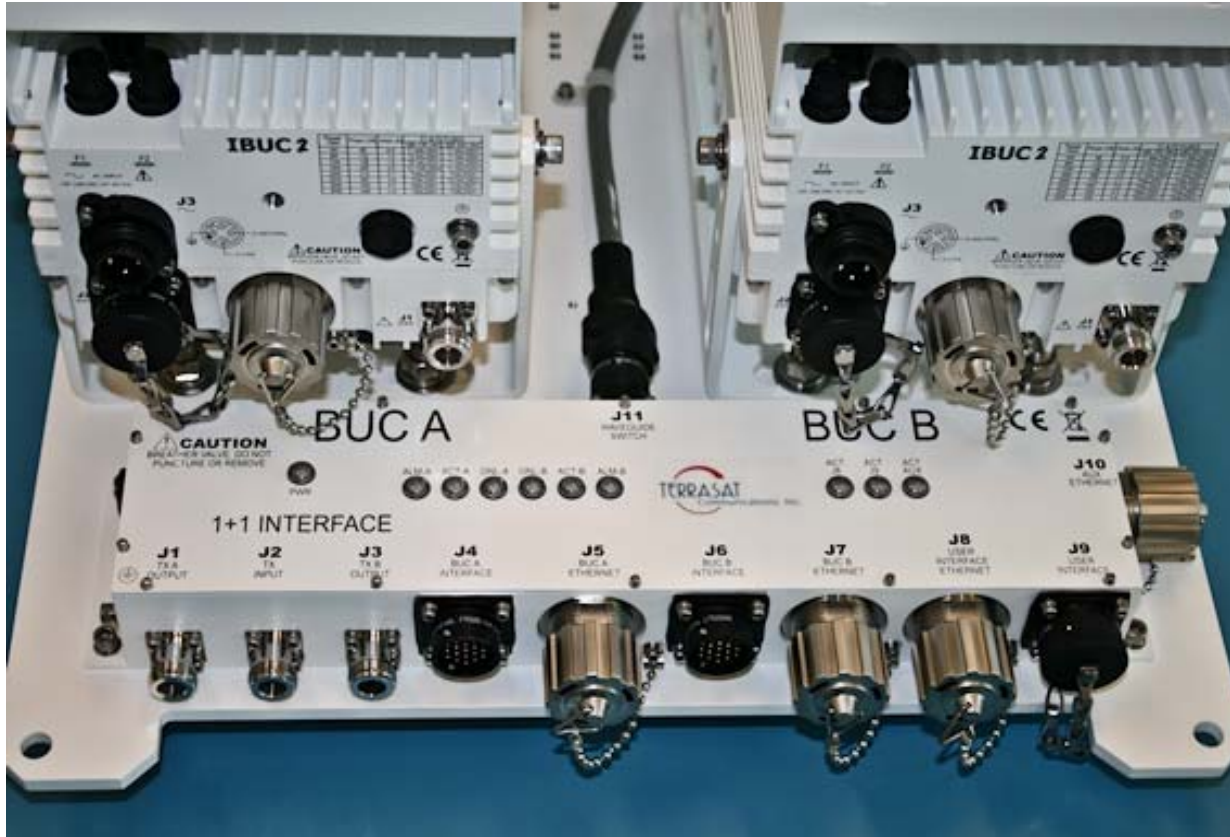
Figure 7.1 Transmit Redundant System Setup
