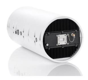
The 200W **TITAN** Ku-Band Block Upconverter is the industry's most compact & lightweight 200W solid state power amplifier. Mission Microwave's proprietary power combining technology and thorough system optimization have produced a rugged 16 lb amplifier that mounts directly on an antenna boom, eliminating excess losses to the feed.
