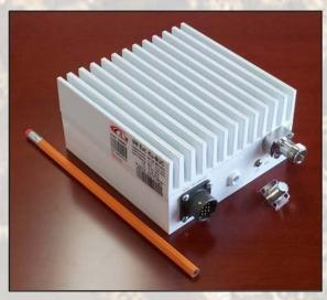
This smallest and lightest 6W L to Ku-Band Block Up Converter is based on GaN technology. Incomparable low power consumption, double L.O., Field-Exchangeable connector and auto-ranging (9 to 36 VDC) powering features make the unit universal for any Ku-Band application. M&C (FSK) capability enables trouble shooting, monitoring and controlling the BUC. User can choose internal 10MHz high stability reference if the corresponding modulator does not provide it.
